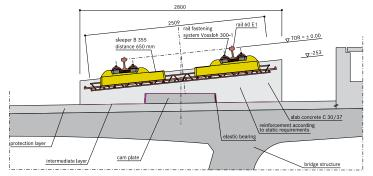
Connection of the track concrete layer with the bridge structure by means of positive cam plates in protection layer
