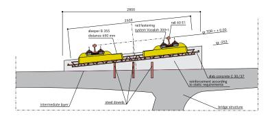
Connection of the track concrete layer with the bridge structure by means of anchor dowels
