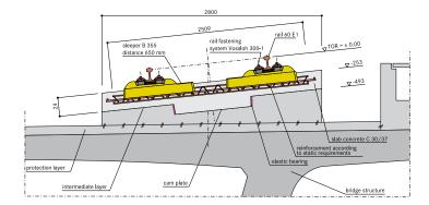
Connection of the track concrete layer with the bridge structure by means of negative cam plates
