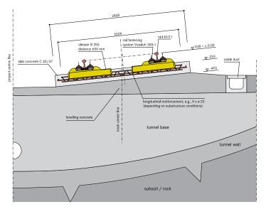
Track concrete layer, installed on levelling concrete
