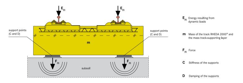
Application of the single-mass oscillator principle in the RHEDA 2000® track type on a mass-spring system
