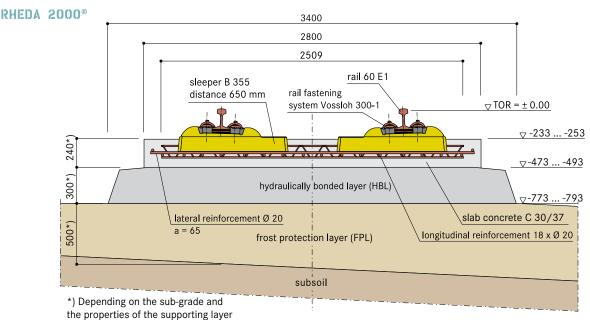
RHEDA 2000<sup>®</sup> is a flexible system that can be individually adapted to the specific requirements and the individual constraints of each project. The basic system structure, however, always consists of modified bi-block sleepers which are securely and reliably embedded in a monolithic concrete slab. Highly elastic rail fastenings are essential to achieve the vertical rail deflection required for load distribution and for smooth train travel.
